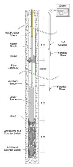
Schematic diagram of an optical fiber borehole strainmeter (graphic by Scott Dewolf).
