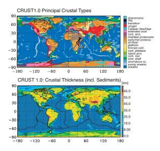
Figure 1: The prototype crustal model CRUST1.0. Top: updated crustal types; Bottom: thickness of the crystalline crust including sediment cover. The input crustal thickness was compiled using existing active source data as we as receiver functions and some gravity data.
