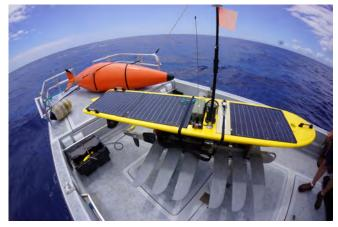
glider in this sea state. The wave glider used in this test was equipped with an auxiliary thruster. When the thruster was running there was approximately a 0.2-0.3 knot speed increase, which nearly compensated for the drag caused by the SHARC.
