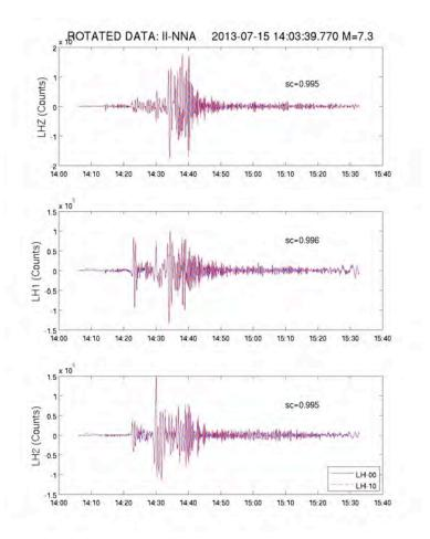
*Figure 2*. Seismograms from a large earthquake recorded on two instruments in Peru. The data from the three orthogonal components (vertical, north and east) nearly match, indicating the instrument responses are known precisely. The response's accuracy is verified with similar tests using Earth tides and normal modes of oscillation.
